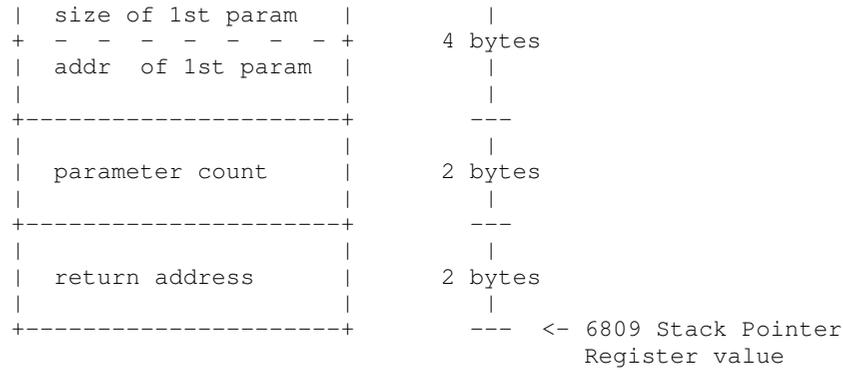
**Figure 9-1. Stack Frame Passed to Machine Language Procedures**
