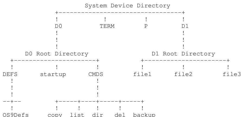
The device names in this example system are "TERM", "P", "D0" and "D1". The root directory of device "D0" includes two directory files, **DEFS** and **CMDs**, and one ordinary file "startup". Notice that device "D1" has in its root directory three ordinary files. In order to access the file "file2" on device "d1", a pathlist having two names must be used:
