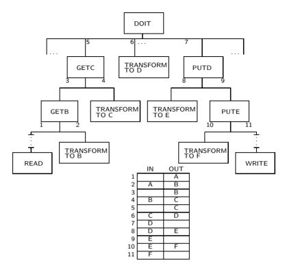
The tiny numbers of the hierarchy chart refer to the lines on the in-out chart. At point 1 (the module READ), the output is the value A. At point 2 (the module TRANSFORM-TO-B), the input is A, and the output is B.
