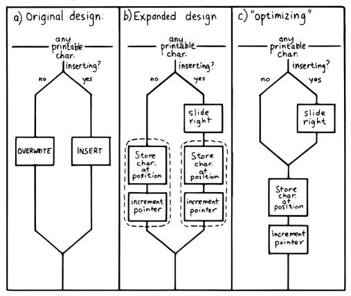
redundancy of code (circled portions). Most competent structured programmers would recognize that this redundancy is unnecessary, and change the structure as shown in Figure 3.6(c). Not too bad so far, right?
