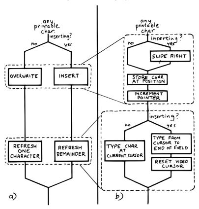
Figure 3.7 (a) shows what happens to our first-pass design when we add refresh. Part (b) shows our "optimized" design with the refresh modules expanded. Notice that we're now testing the Insert flag twice within this single leg of the outer loop.
