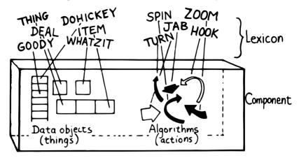
Suppose that, after the program is written, we need to change the record structure. In the sequential, hierarchical design, this change would affect all three modules. In the design by components, the change would be confined to the record-structure component. No code that uses this component needs to know of the change.
