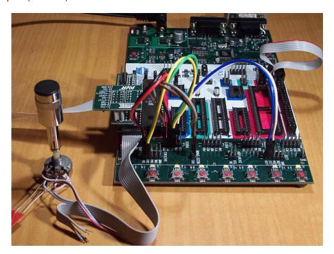
Figure 6: Setup of the STK500
