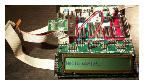
Figure 9: Wiring of the STK500
